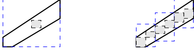
Figure 5. A worst-case scenario for over- and under approximation by a single hypercube (left) and a less pessimistic over- and under approximation using many hypercubes.
